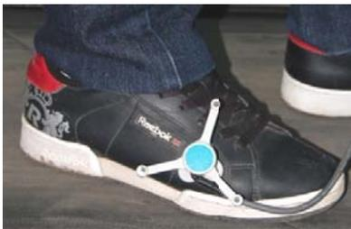
**Figure 1: Zebris CMS-HS measuring system**
