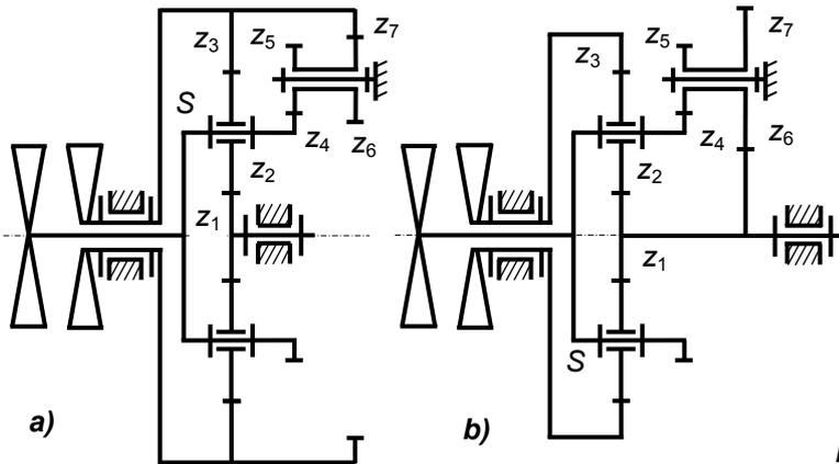
**Fig. 2. Closed differ. reducers for coaxial propellers**
