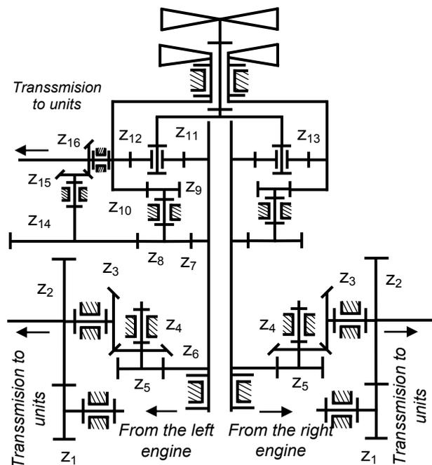
**Fig. 6. Kinematic scheme of the reducer RV-3F from the helicopter Kamov Ka-25K**
