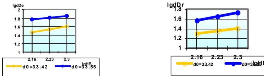
**Fig. 3 The influence of the material's hardness on the outer diameter and on the diameter over the rolls**
