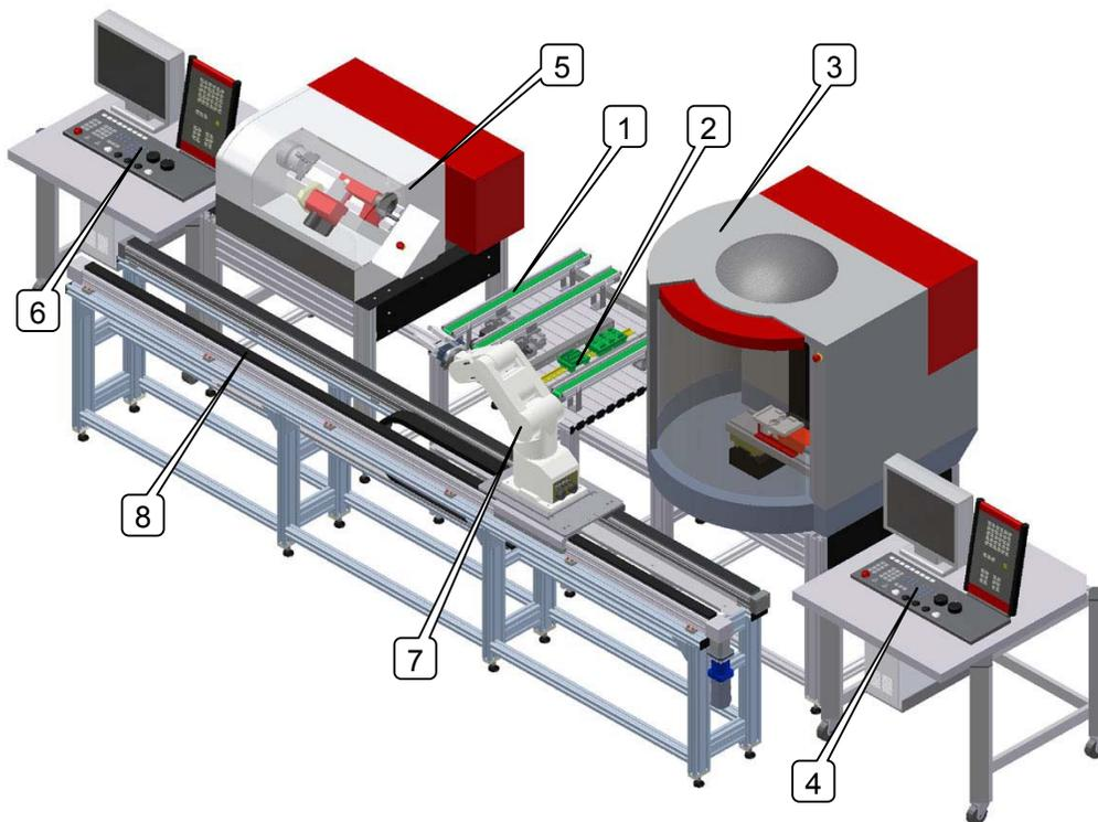
**Figure2 A007 Flexible manufacturing system**
