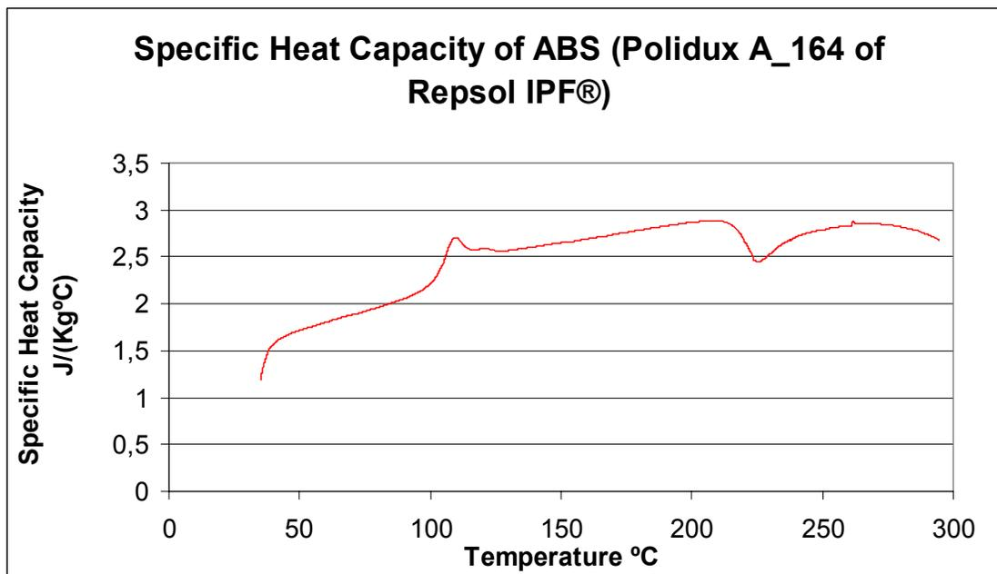
**Figure 3. Cp ABS (Polidux A\_164 of Repsol)**
