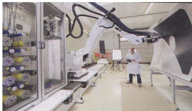
Fig.2. Robot system lays thermoset, thermoplastic or dry fiber [2].
