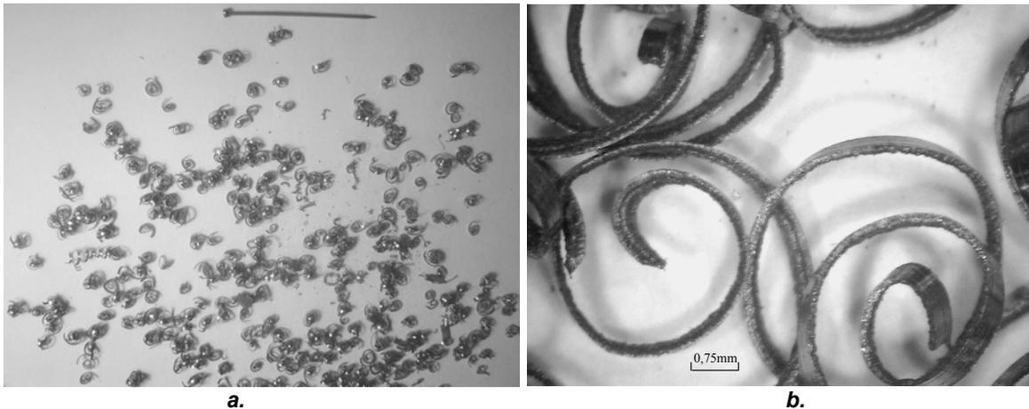
**Fig.5 – Chips forms resulted at turning with a cutting feed of  $f = 0,088$  mm/rot**
