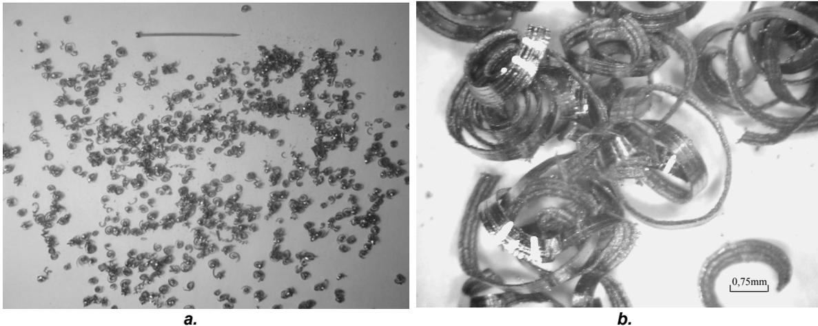
**Fig.1 – Chips forms resulted at turning with a cutting feed of  $f = 0,053$  mm/rot**
