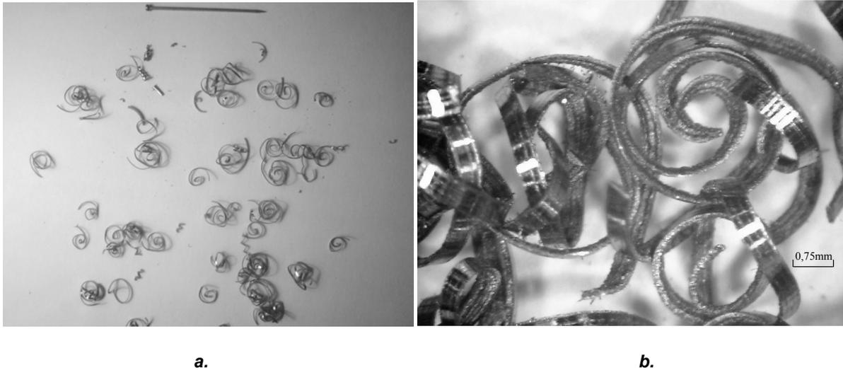
**Fig.4 – Chips forms resulted at turning with a cutting feed of  $f = 0,083$  mm/rot**
