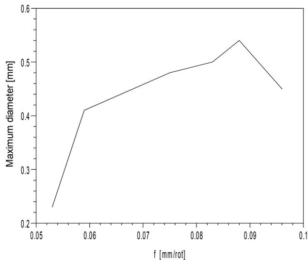
**Fig.7 Dependency of chip diameter upon cutting feed**
