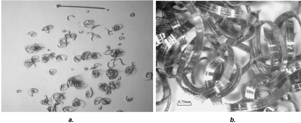
**Fig.3 – Chips forms resulted at turning with a cutting feed of  $f = 0,075$  mm/rot**
