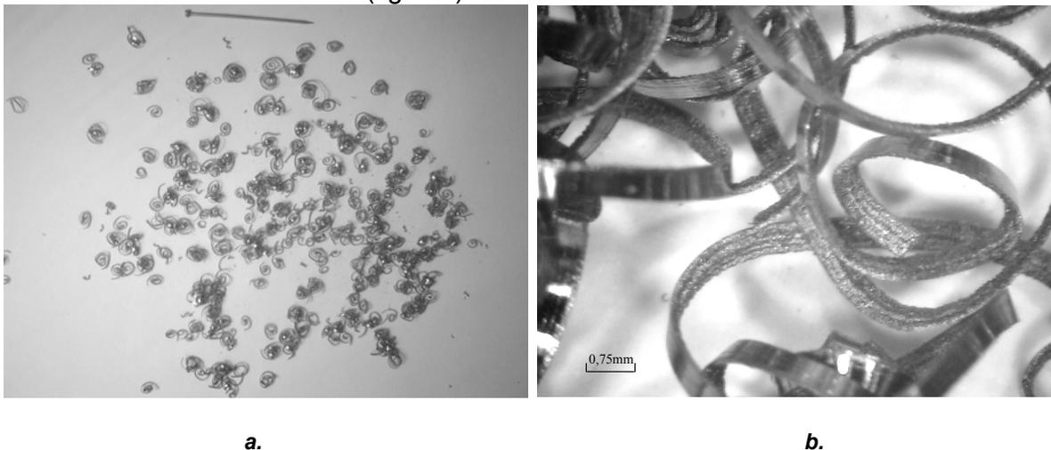
**Fig.6 – Chips forms resulted at turning with a cutting feed of  $f = 0,096$  mm/rot**
