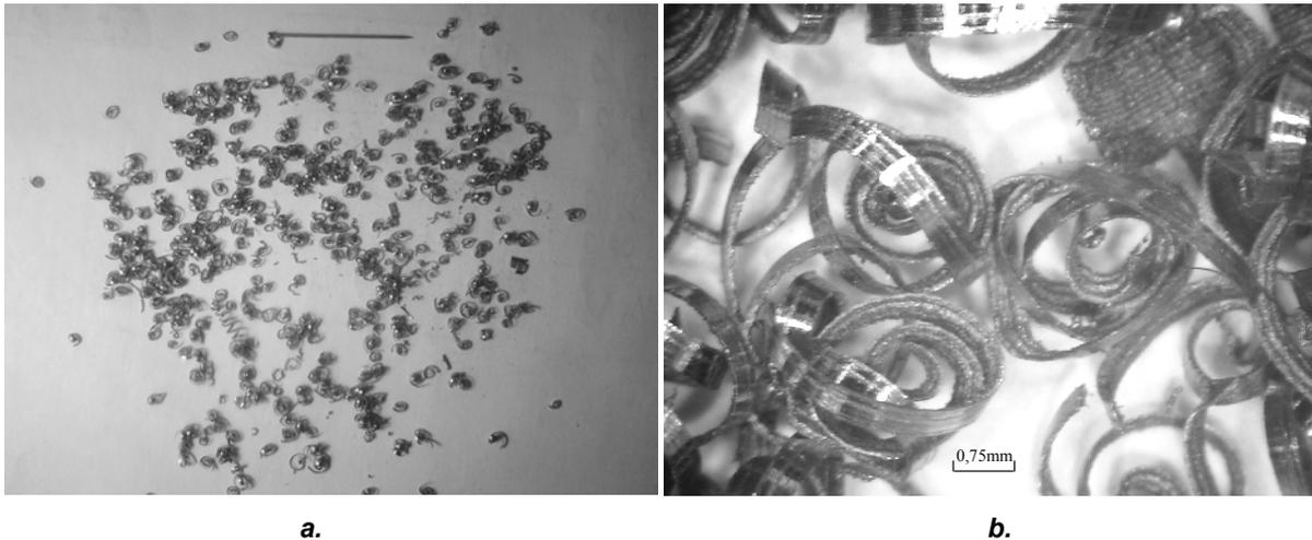
**Fig.2 – Chips forms resulted at turning with a cutting feed of  $f = 0,059$  mm/rot**
