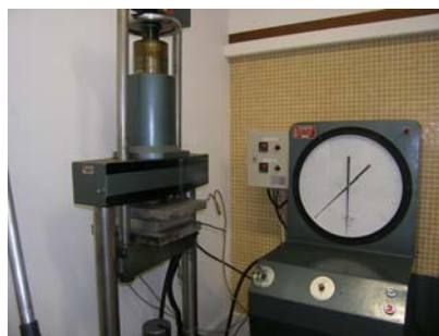
Figure 6. Hot plate press used.
