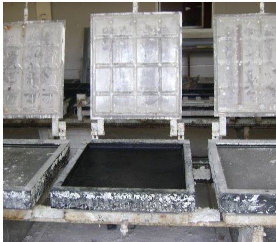
Fig.4. The mold of casting and the inner designer of mold [4].
