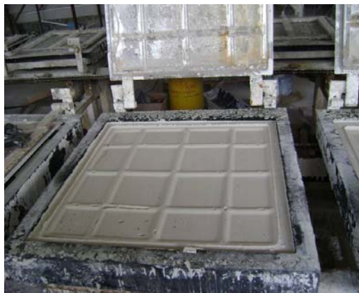
Fig.5. The sound-absorbing panel inside of mold casting [4].
