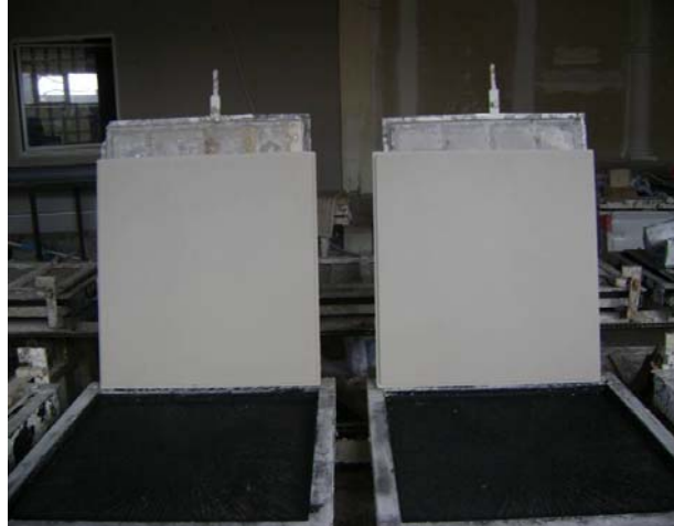
Fig.6. The mold and taken out of panel from modeling plaster [4].
