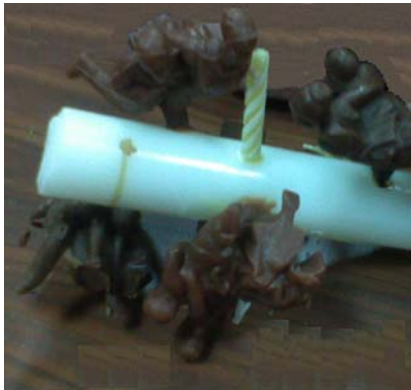
Fig.7 Wax tree assembly, TUCN
