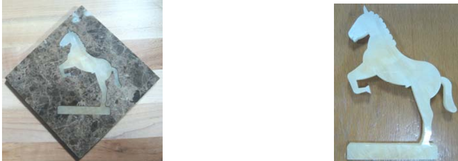
Fig.10 The part made from marble whit 15mm thickness
