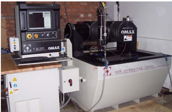
Fig.7 The AWJ equipment, Omax 2626, Technical University of Cluj-Napoca, TUCN
