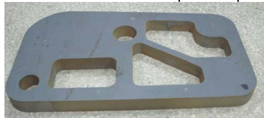
Fig.9 The part made from Steel OL52 with 20mm thickness
