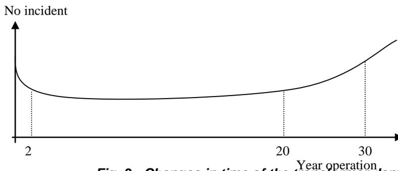
**Fig. 3. Changes in time of the transformer damage**
