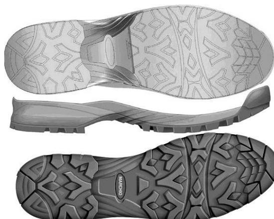
**Figure 3. Design of anti-skid pattern**
