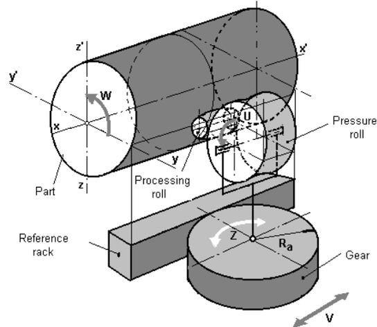
**Fig. 3. Basic diagram of the vibro-rolling using a convex-profile roller**
