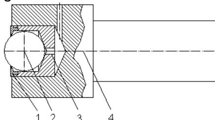
**Figure 7. Common rolling head. 1. retainer ring; 2. ball; 3. anti-friction part; 4. Frame**
