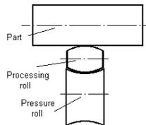
**Fig. 4. Chart representing the processing operation**
