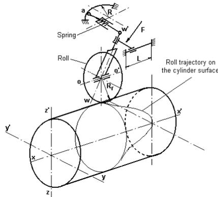
**Figure 5. Short presentation of the device; the roller impression on the part is a sine curve**
