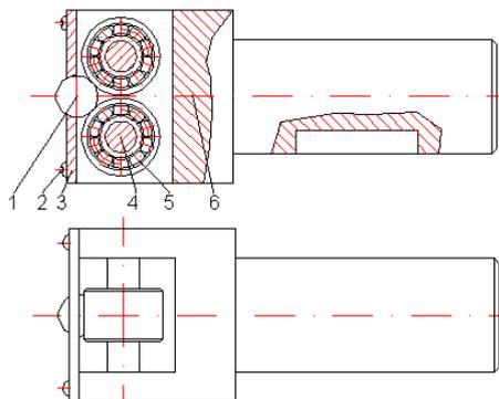
**Fig.1. Rolling head used for the vibro-rolling device: 1. rolling ball; 2. screw for temple clamping; 3. temple; 4. shaft; 5. rolling bearing; 6. fork**
