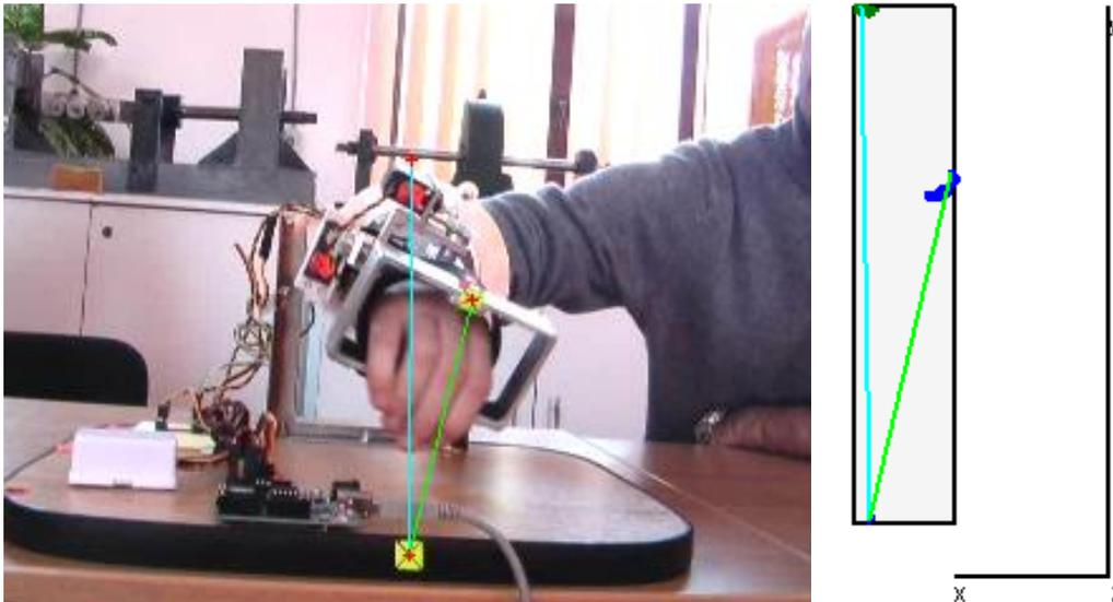
Figure 8. Pronation/supination motion analysis performed by the robotic system using SIMI Motion equipment
