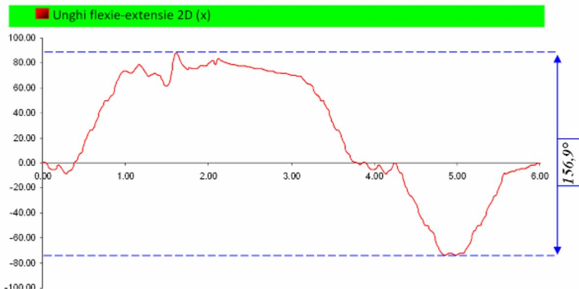
Figure 9. Flexion/Extension angular amplitude developed by using this robotic system
