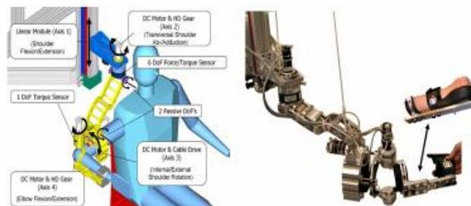
**Figure 1. ARMin exoskeleton for human upper limb recovery**
