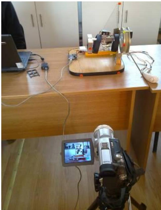
**Figure 3. SIMI Motion analysis equipment and the installing mode onto proposed robotic system**
