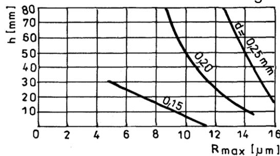
**Fig.11. Roughness of worked surface; copper wire-electrode, steel part-electrode.**
