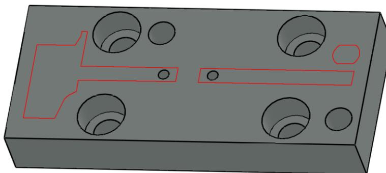
**Fig.4.b. Die active part, after milling and boring.**
