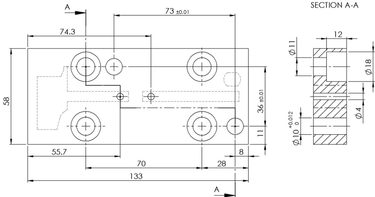
**Fig.4.a. Execution drawing of the die active part.**
