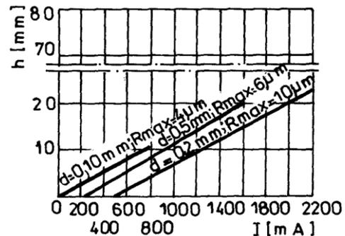
**Fig.8. Choice of working current according to the material to be worked; copper wire-electrode, steel part-electrode.**
