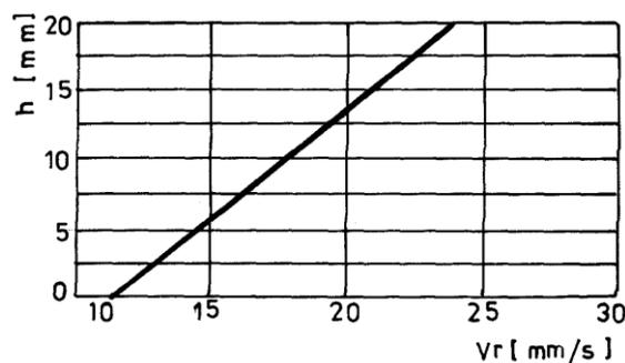
**Fig.6. The electrode rolling speed  $v_r$  versus the thickness of the worked part  $h$ .**
