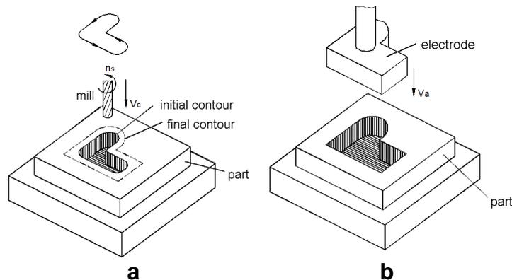
**Fig.2. Working of blind-end complex surfaces: a – by milling, b – by EDM.**
