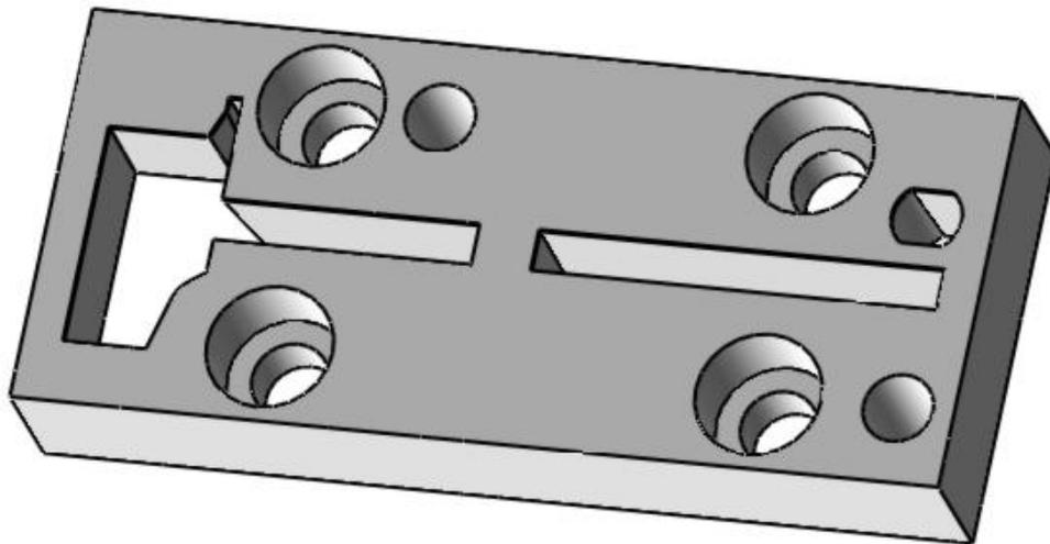
*Fig.12. Finished die active part, after wire-electrode EDM.*
