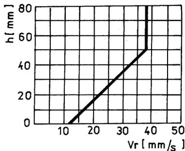
**Fig.7. Choice of the rolling speed according to the material to be worked; copper wire-electrode, steel part-electrode.**
