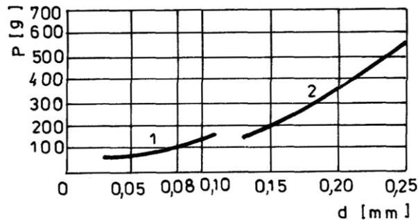
**Fig.5. Tensile force  $P$  versus wire-electrode diameter  $d$ ; 1 – hard copper, 2 – soft copper.**
