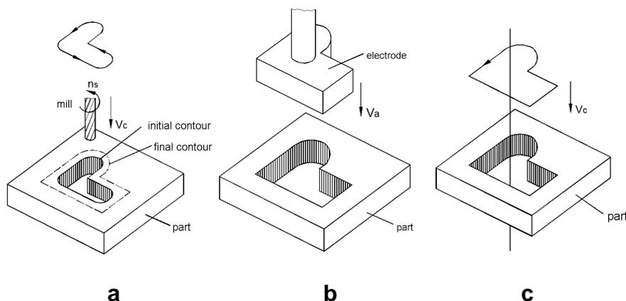
**Fig.1. Working of complex through-hole surfaces:
