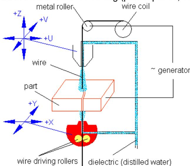
**Fig.3. Working principle of wire EDM installation.**
