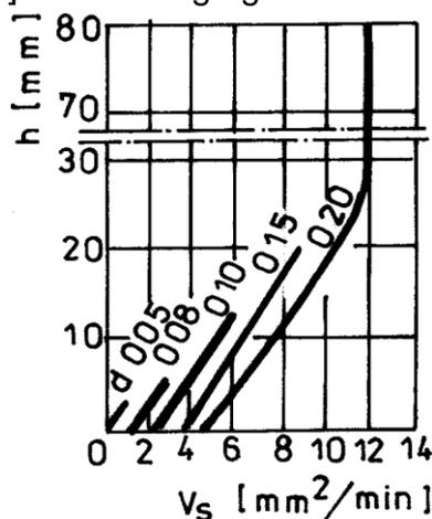
**Fig.9. Cutting capacity according to the material to be worked; copper wire-electrode, steel part-electrode.**
