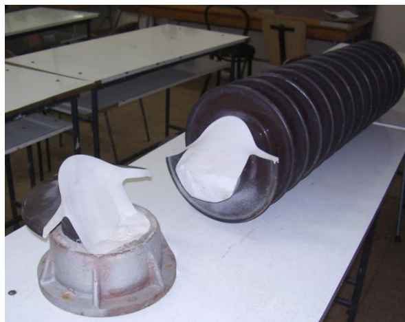
Fig.1.2. Ceramic Insulator broken from the metallic bottom support
