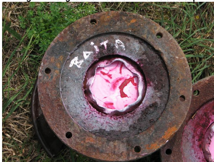
Fig.2.5. Deep crack on the base of the ceramics body.
