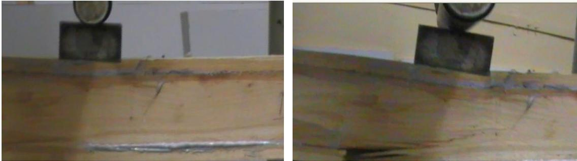
**Fig.3 Up and down reinforcement application: two sheets of composite material**
