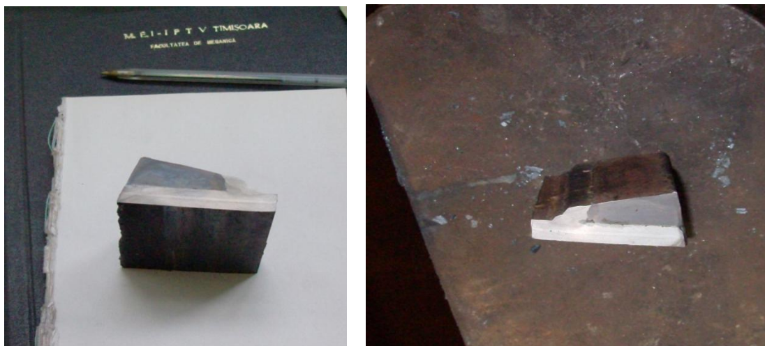
Fig.6. Macroscopic appearance of the weld
