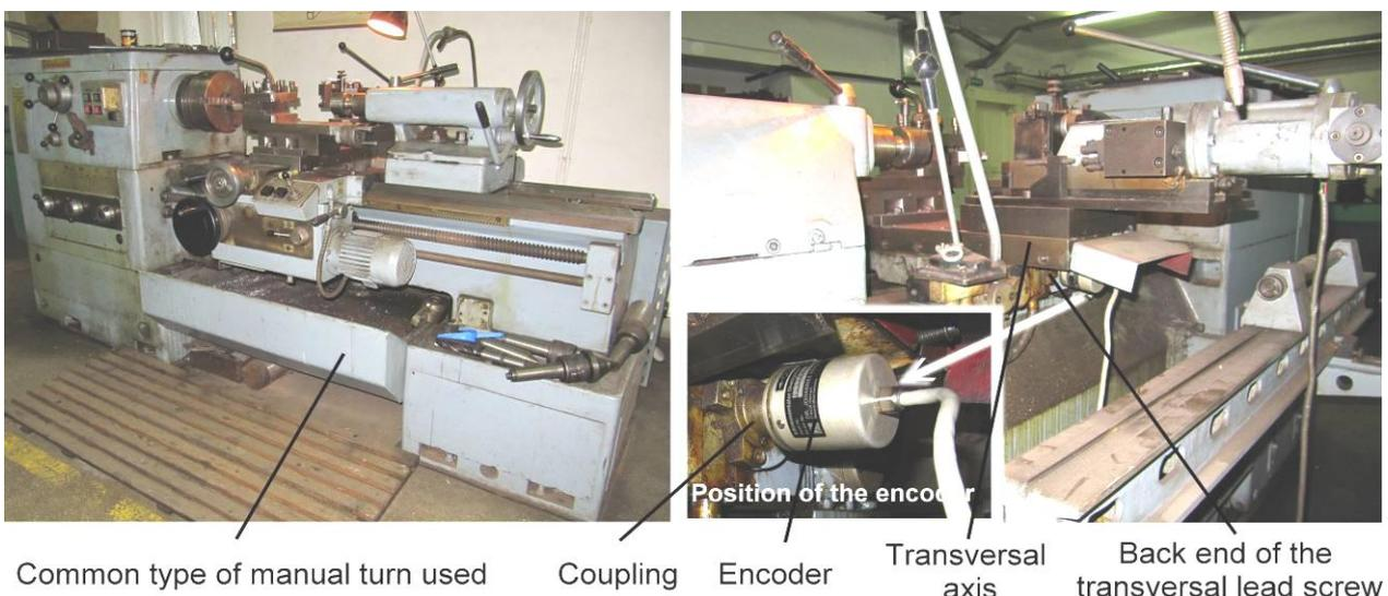
**Figure 2. Common type of lathe used for the application with added optical rotary encoder**
