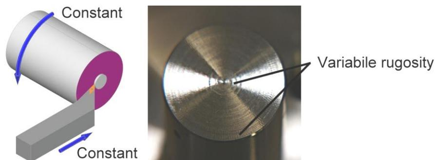
**Figure 1. The fix rotation speed creates variable rugosity**
