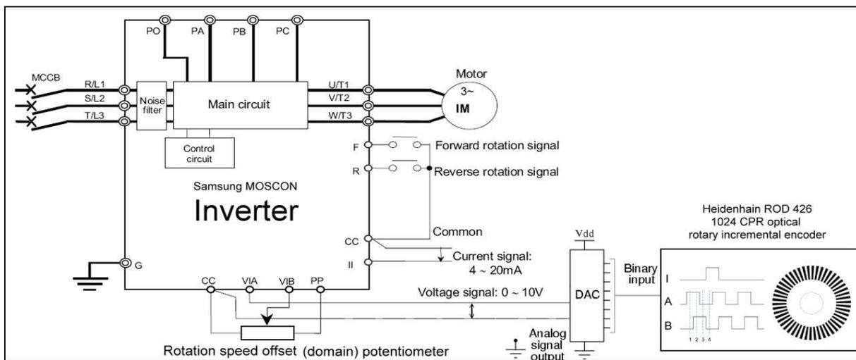
**Figure 4. Schematics of the installation**
