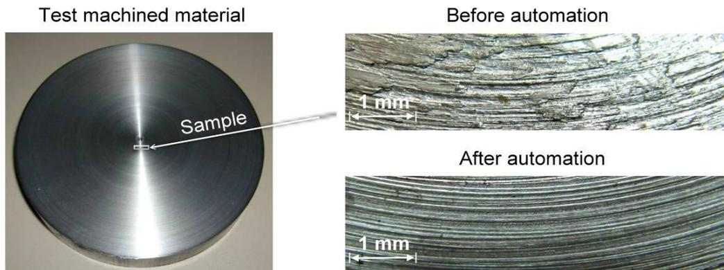
**Figure 5. The resulted comparative surface after automation**
