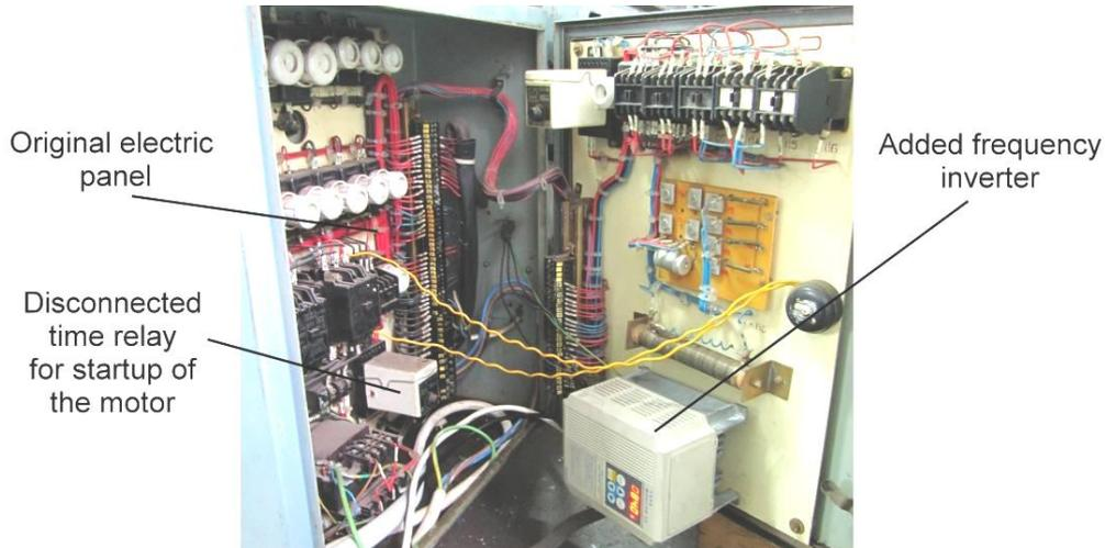
**Figure 3. In the original electric box a proper frequency inverter is coupled to the existing installation**
