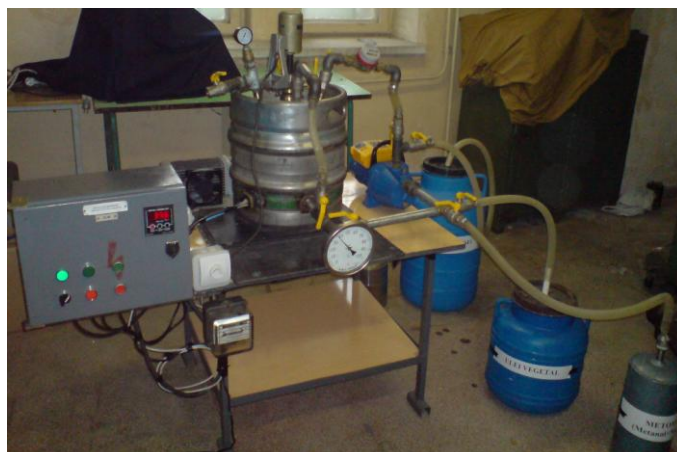
Fig.2 Experimental installation for biodiesel production
