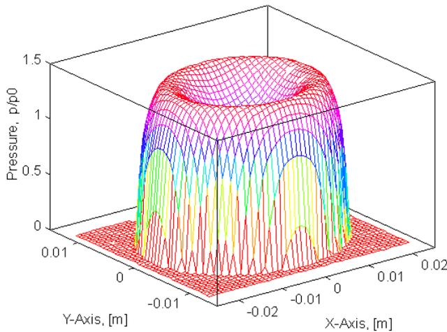
**Figure 1. Pressure distribution on elliptic contact area**
