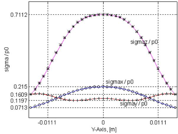
**Figure 6. Normal stresses along minor axis**
