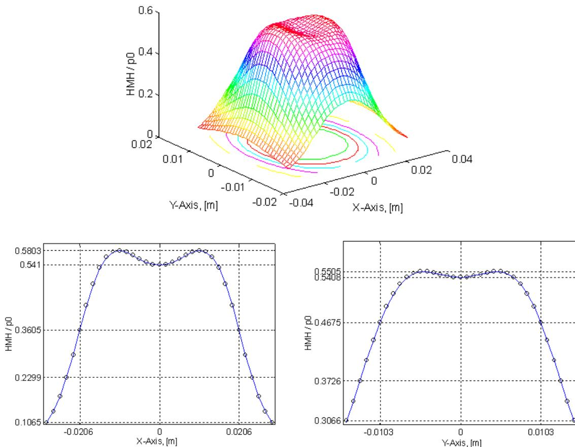
**Figure 7. Equivalent von Mises stress at depth  $z = 0.8b$**
