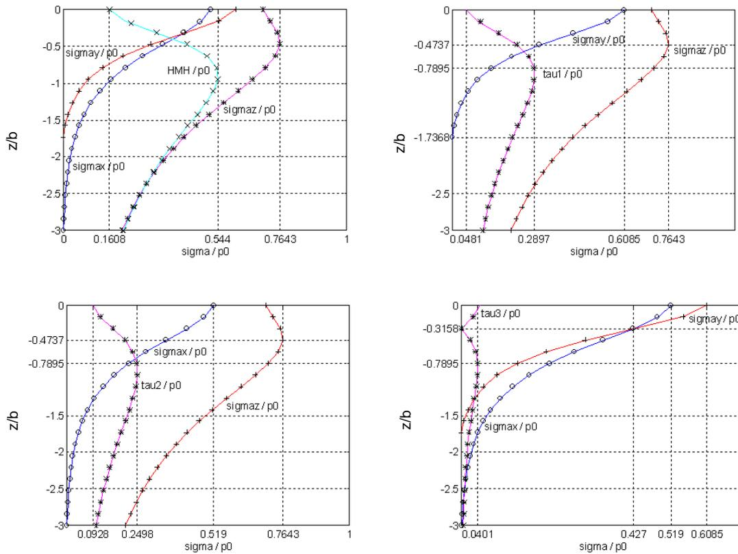
**Figure 8. Stress components on the central axis of the contact**
