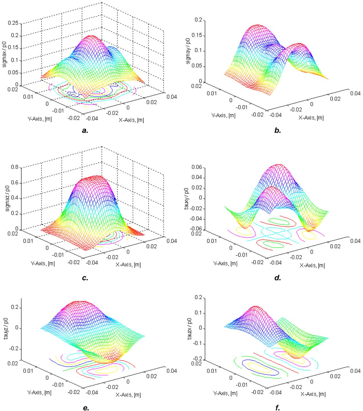
**Figure 4. Contact stresses at depth  $z = 0.8b$**
