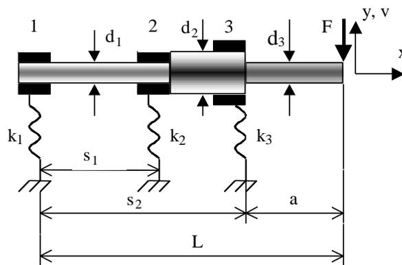
**Figure 1 Beam on three bearings**
