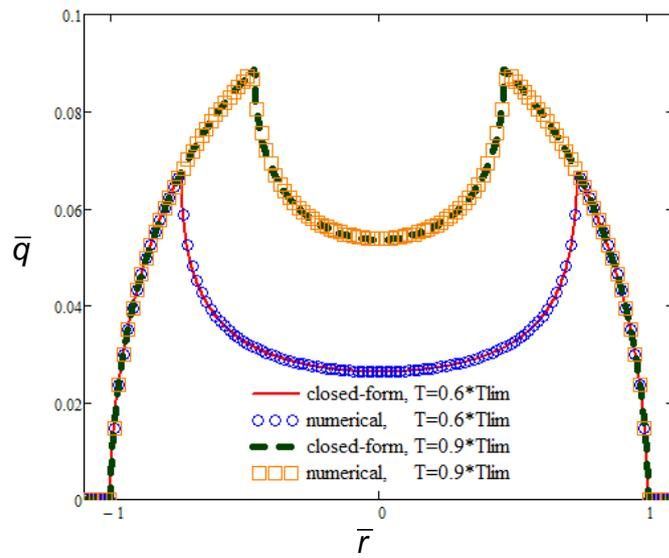
**Figure 2. Dimensionless shear stress profiles in the plane  $y = 0$**
