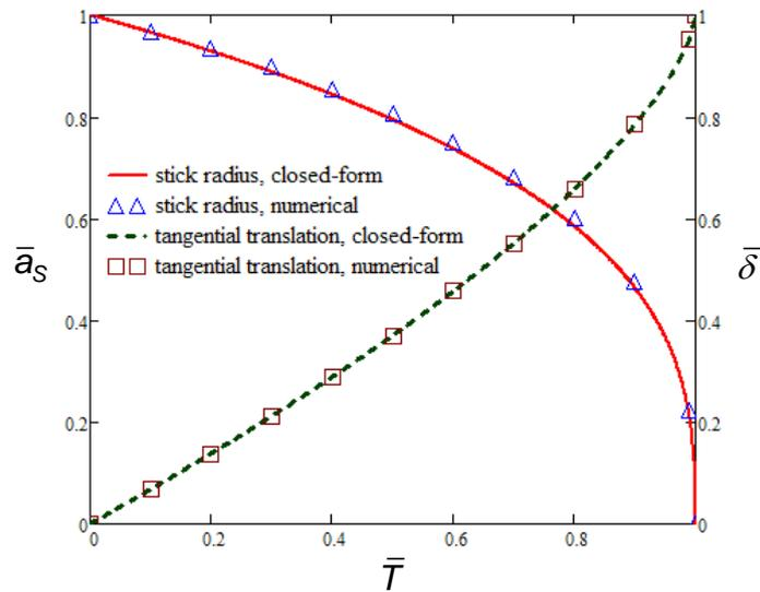
**Figure 3. Dimensionless stick radius and tangential displacement versus loading level**
