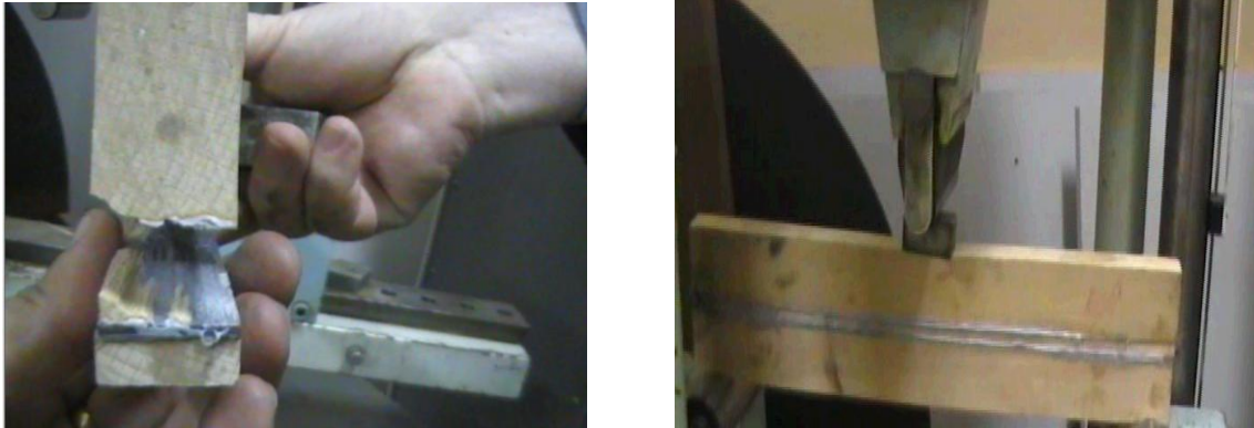
Fig. 3 Tension failure of a reinforced wood beam with three CFRP sheets
