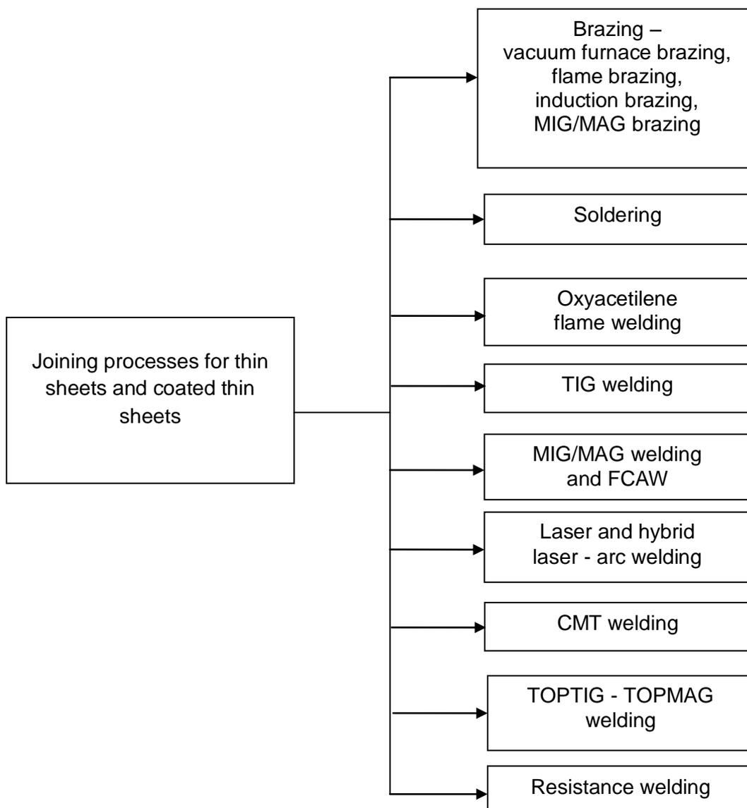
**Figure 1. Schematic representation of joining processes for thin sheets and coated thin sheets**
