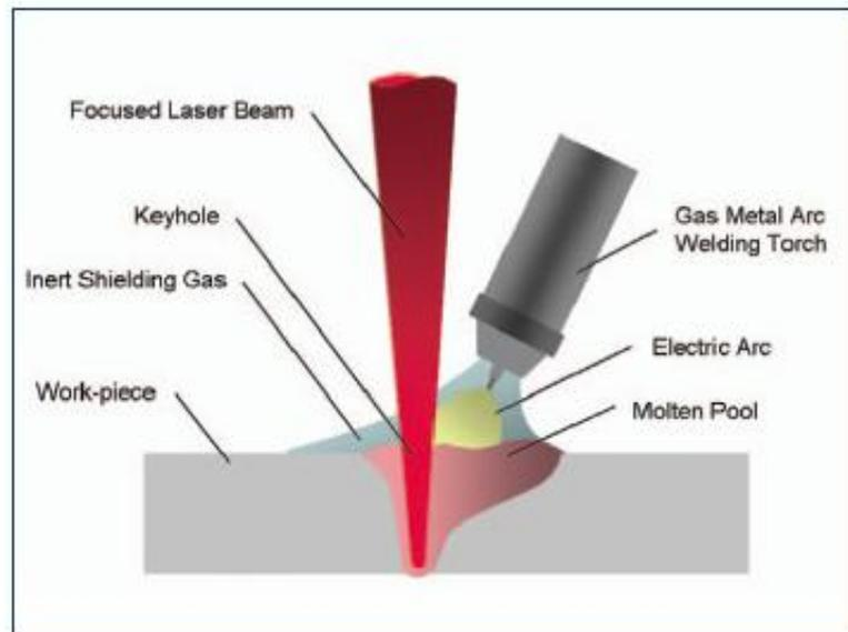
Figure 2. Hybrid laser arc welding process (laser leading) [4]
