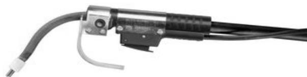
K126- 350 Ampers at 60% DA, wire diameter 1.6-2.4 mm
