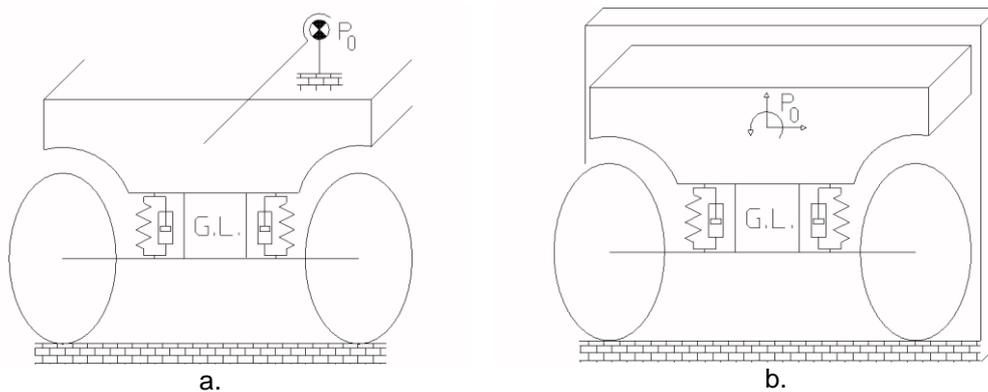
**Figure 2. Half-car models to evaluate the roll motion (G.L. - guiding linkage)**
