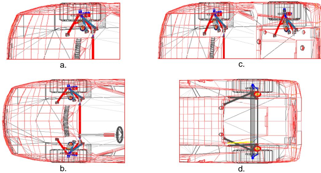
**Figure 1. Suspension assemblies (quarter-car and half-car models)**
