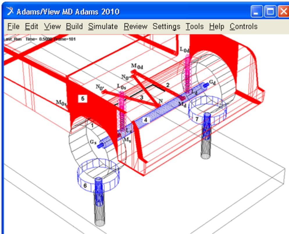
**Figure 3. The MBS dynamic model of the rear axle suspension system**
