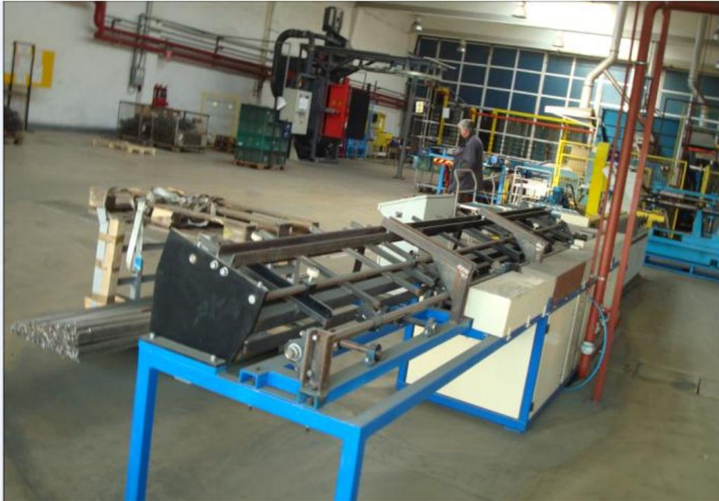
*Fig. 1. Machine from the S.C Compa Sibiu which produces the heating of the bar through the induction process*
