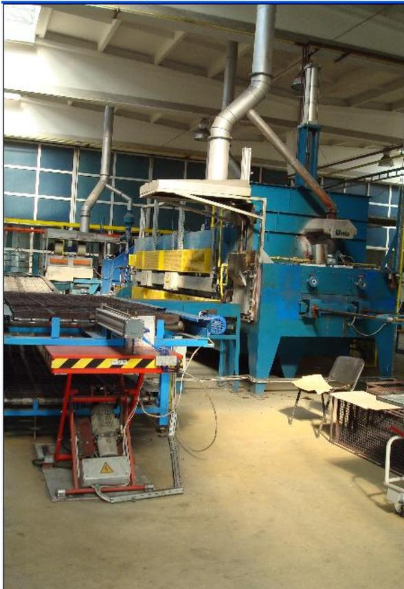
**Fig.3. Machine for spring-hardening heat treatment**
