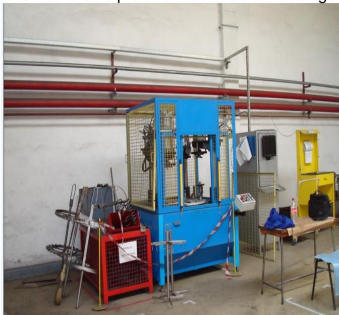
**Fig.5. Machine for BLOCK compression**
