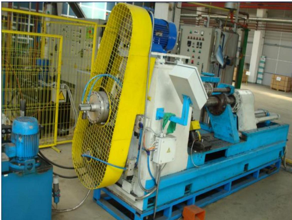
*Fig.2. Machine wrapped mandrels*
