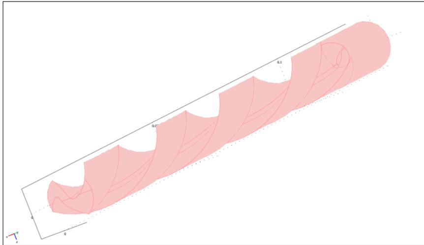
**Fig. 1.** Geometrical 3D model of the drill body.
