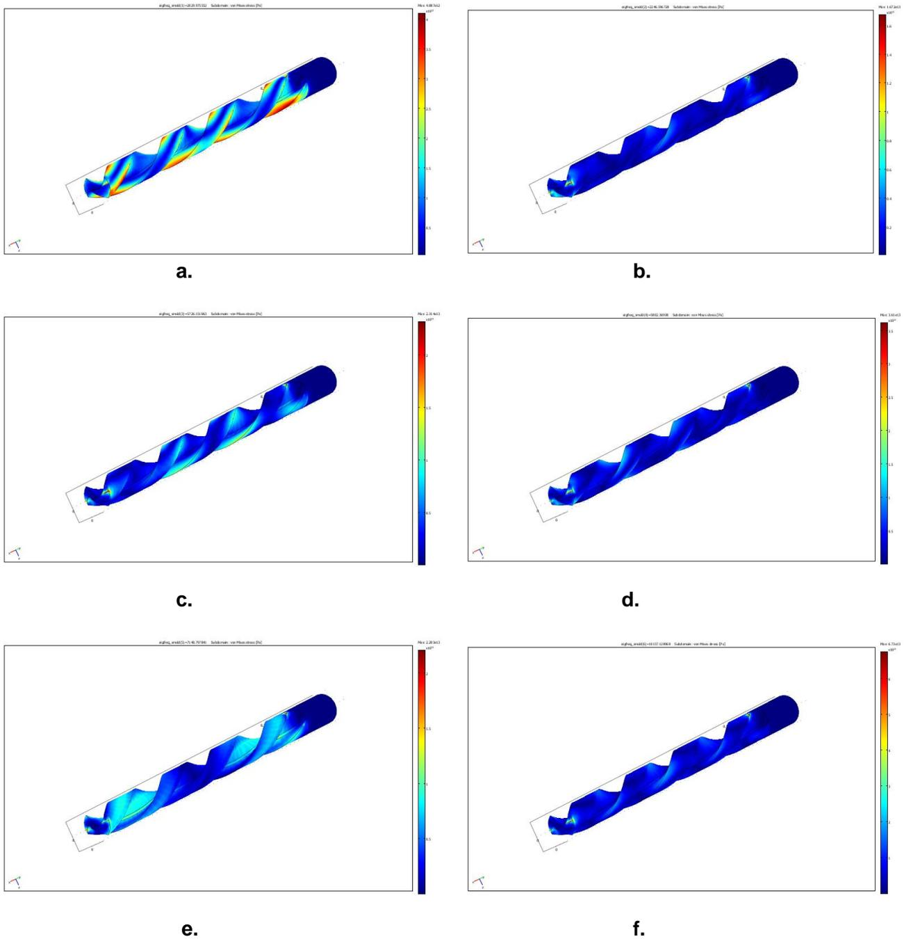
**Fig. 3.** 3D finite element analysis results (von Mises stress) for 6 major natural modes: a. 2029 Hz; b. 2246 Hz; c. 5726 Hz; d. 5802 Hz; e. 7140 Hz; f. 10137 Hz .
