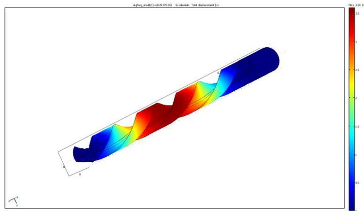
**Fig. 4.** 3D finite element analysis of the drill total displacement for the natural frequency of 2029 Hz..
