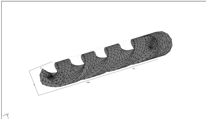
**Fig. 2.** 3D finite element mesh model of the drill body.
