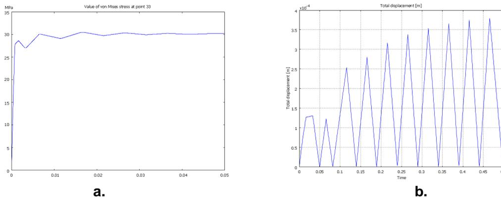
**Fig. 6.** Result diagrams for central point of the drill: a. von Mises stress diagram as function of time for impact load; b. total displacement diagram as function of time for load defined by expression [1].
