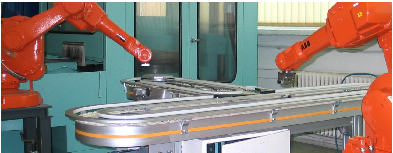
Fig. 5 FlexLynk conveyor served by the two ABB robots.
