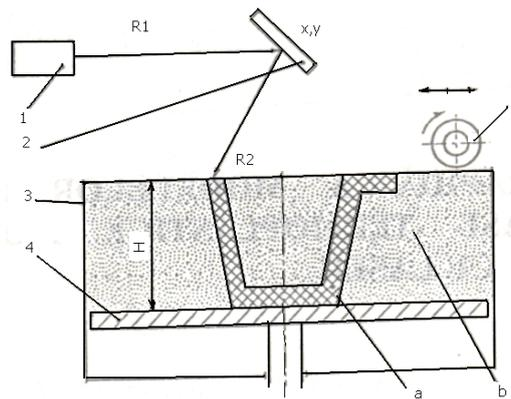
**Fig. 1. Laser sintering operation is shown schematically in figure 1 - laser, 2 - scanner, 3 - tank, 4 - mobile platform, 5 - smoothing and drying system, R1, R2-ray laser-part consists of b-powder.**
