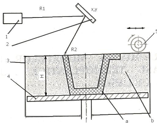
**Fig. 1. Laser sintering operation is shown schematically in figure**
