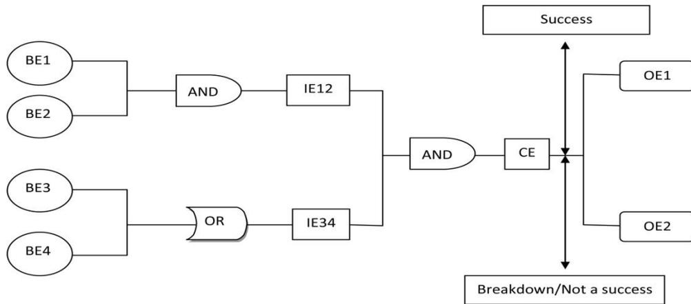
**Fig. 1 Elements of a "Bow-tie" diagram**
