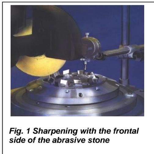
*Fig. 1 Sharpening with the frontal side of the abrasive stone*
