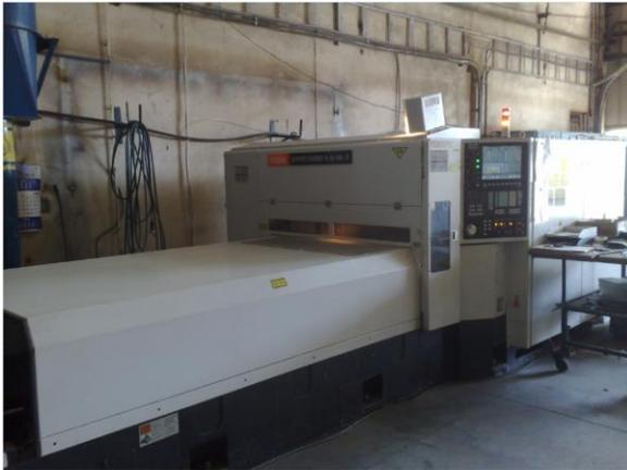
**Figure 2. Laser system Mazak Super Turbo-X 48 Mk2 1800W**
