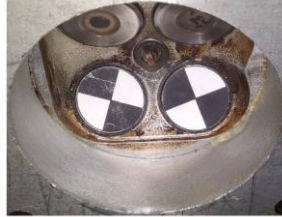
Figure 3. The markers positioned on exhaust valve heads
