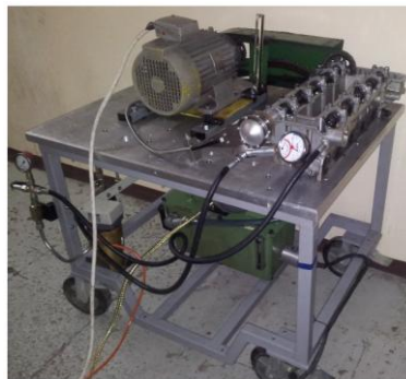
Figure 2. Test rig used for measuring the valve rotation
