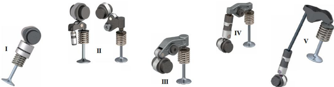
Figure 1. Types of valve train: I direct acting; II end pivot rocker arm; III center pivot rocker arm; IV center pivot rocker arm with follower; V pushrod.
