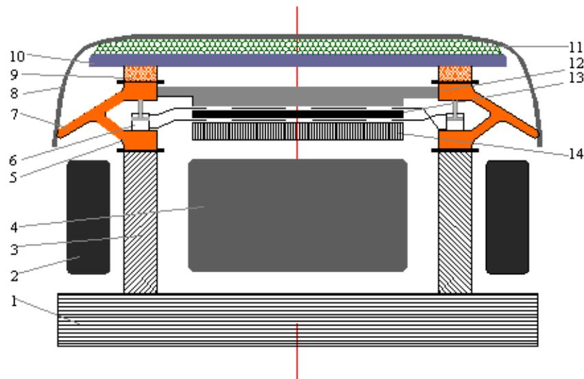
**Figure 9. Adaptive structure for frontal collisions: 1-firewall, 2-wheel, 3-longitudinal member, 4-engine, 5-adaptive part, 6-hidraulic cylinder, 7-deflecting device, 8-bumper, 9-collapse member, 10-transversal member, 11-shock absorber, 12-tragger, 13-AC condenser, 14-cooler**
