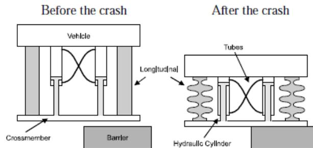
**Figure 6. A hydraulically controlled frontal car**
