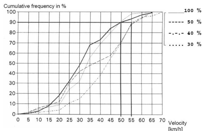
**Figure 1. Cumulative frequency of velocities in frontal collisions (source: Justen 1993).**
