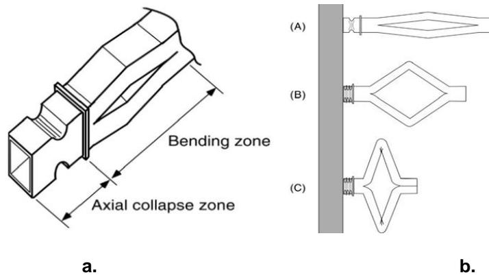
**Figure 5 a. Fundamental model of a crash load control structure (Motozawa, Kamei)**
