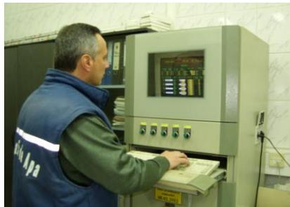
**Figure 2. Metrological verification of water meters [1]**
