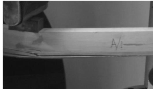
**Figure 2 Tension failure of a reinforced beam with carbon fiber plates [3,4]**
