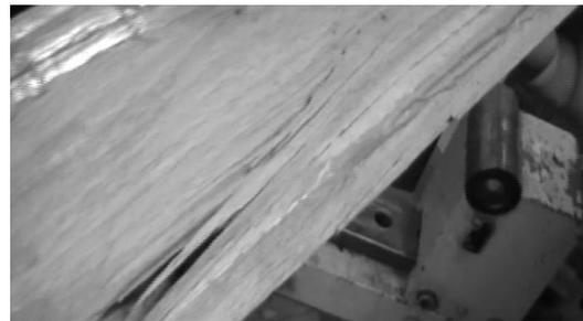
**Figure 1 Tension failure of a reinforced beam with carbon fiber sheet [3,4]**
