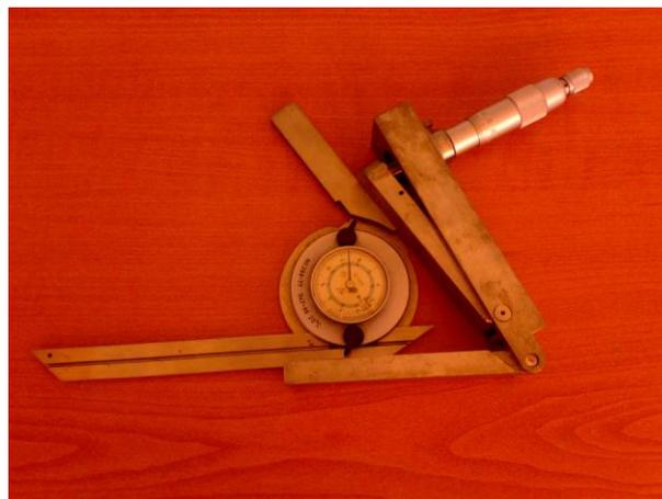
**Figure 7: Testing portable adjustable sine ruler**
