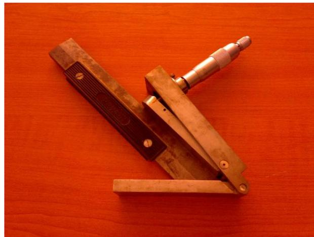
**Figure 9: Measuring method using portable adjustable sine ruler**
