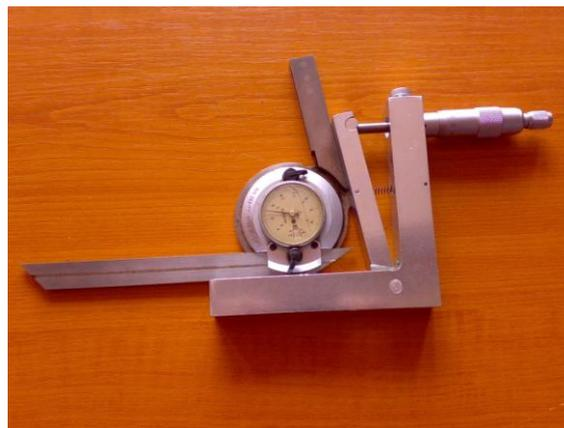
**Figure 3. Testing the non-adjustable portable sine rule**
