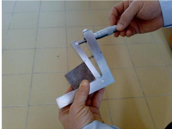
**Figure 5. Non-adjustable portable sine rule measurement methodology**
