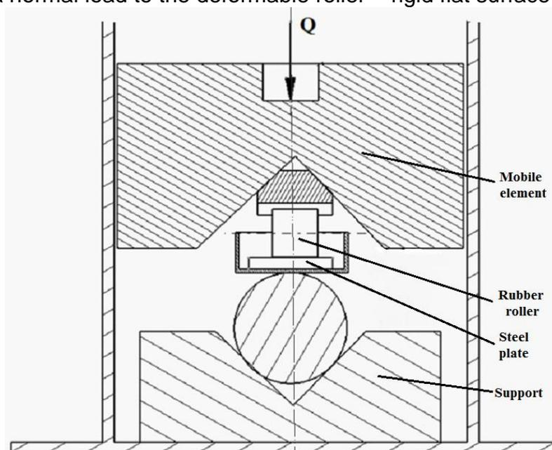
Figure 1. Schematic representation of the device used to investigate line contacts
