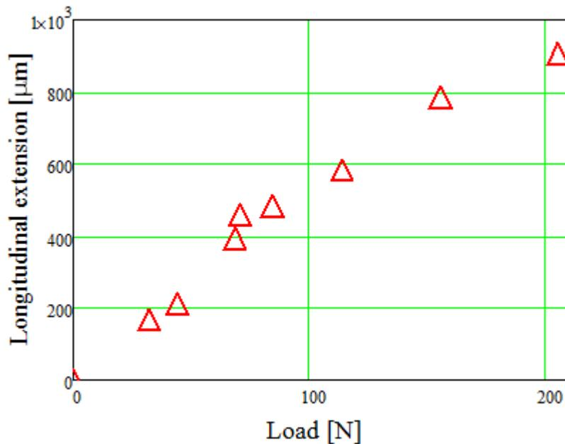
**Figure 7. Correlation between contact area longitudinal extension and load for a cylindrical rubber roller with  $\Phi = 20\text{mm}$ , and  $l = 11.4\text{mm}$ , pressed against a flat steel plate**
