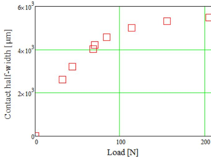
**Figure 6. Contact half-width variation with normal load, for a cylindrical rubber roller with  $\Phi = 20\text{mm}$ , and  $l = 11.4\text{mm}$ , pressed against a flat steel plate**
