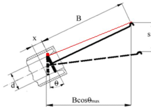
**Figure 6 The tangential mechanism**
