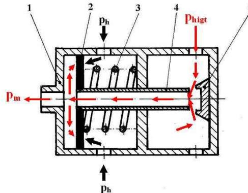
**Figure 3 The first stage pressure regulator of the emergency reservoir**
