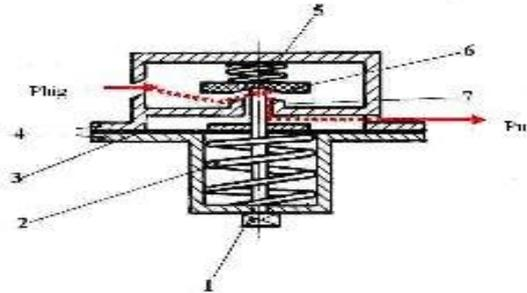
**Figure 1 The regulator of the main reservoir from the surface**
