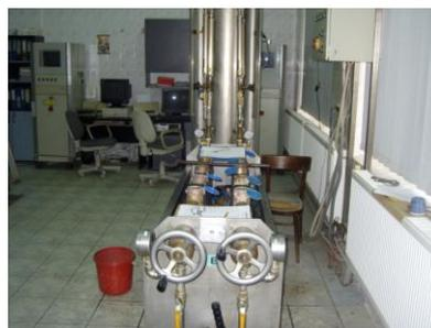
*Figure 4. Metrological verification stand of water meters [1]*
