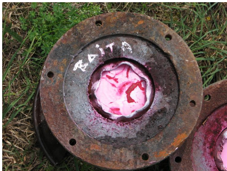
Fig.4.5 Deep crack on the base of the ceramics body.
