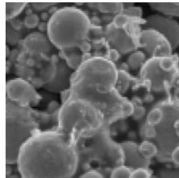
**Fig.2. Al<sub>2</sub>O<sub>3</sub> particles (99.5%), sintered by laser beam on the surface OLC45 (electronic 1500x).**
