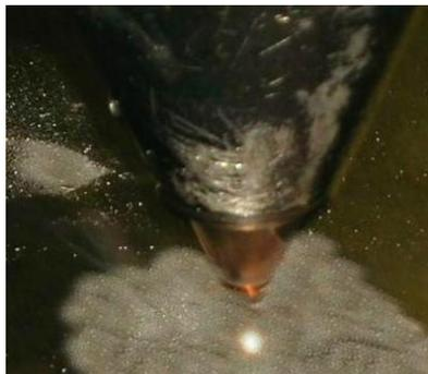
**Fig. 1. Deposition on the surface of a piece of 4mm thick material OLC45.**
