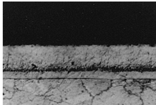
*Fig.4. Deposition of powder  $\text{Al}_2\text{O}_3$  (99,5%) on the support OLC 45 (thickness deposited  $h = 0,6\text{ mm}$ , optic 100x)*
