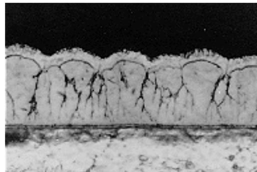
*Fig.6. Deposition of powder  $\text{Al}_2\text{O}_3$  (99,5%) on the support OLC 45 (thickness deposited  $h = 1,2\text{ mm}$ , optic 100x)*
