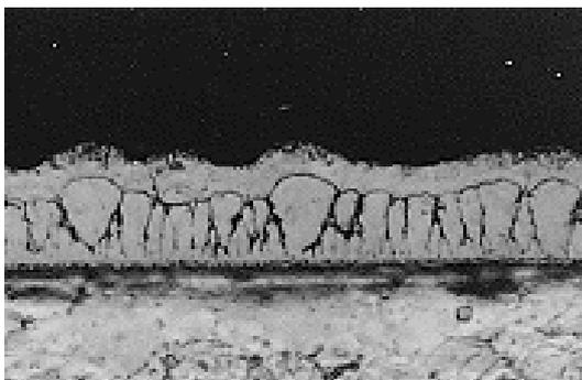
*Fig.5. Deposition of powder  $\text{Al}_2\text{O}_3$  (99,5%) on the support OLC 45 (thickness deposited  $h = 1\text{ mm}$ , optic 100x)*
