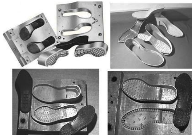
Figure 4. Moulds with interchangeable cavity with two cavities
