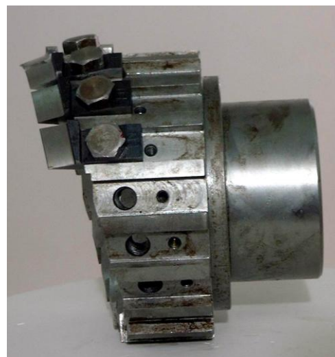
Fig.4 Technological device equipped with grinded cutters
