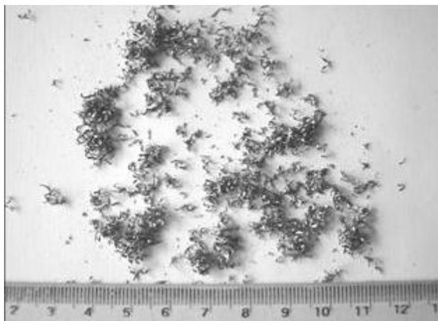
**Fig.20. Chips resulted after mill-end of sample 3**
