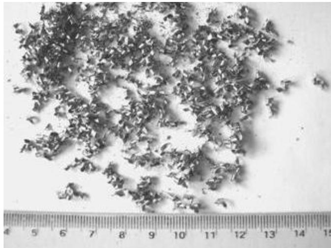
**Fig.10. Chips resulted after mill-end of sample 7**
