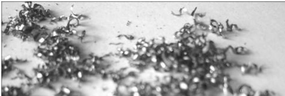
**Fig.17. Chips resulted after mill-end of sample 15**
