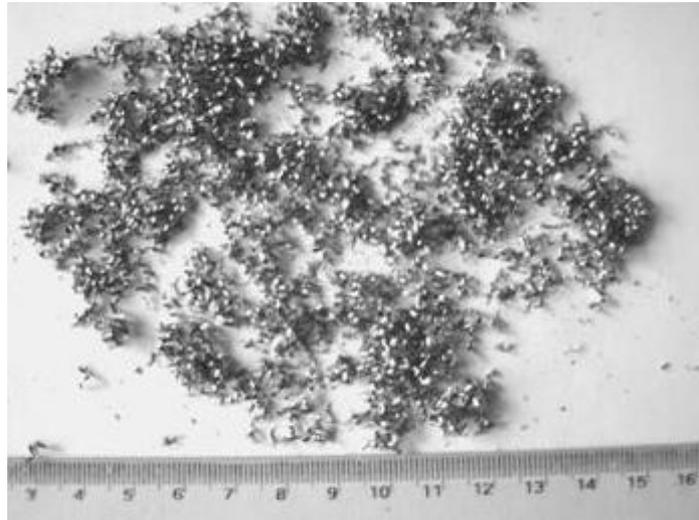
**Fig.12. Chips resulted after mill-end of sample 9**
