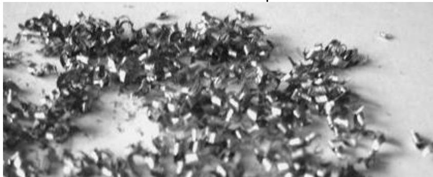
**Fig.11. Chips resulted after mill-end of sample 8**
