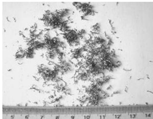
**Fig.21. Chips resulted after mill-end of sample 4**
