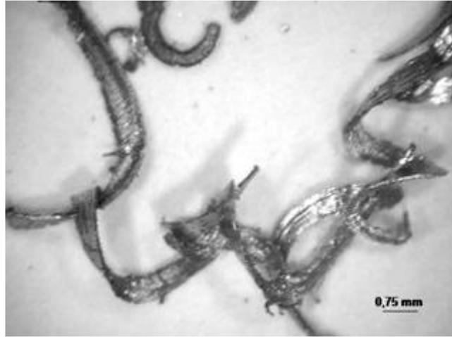
*Fig.22. Chips resulted after mill-end of sample 13*
