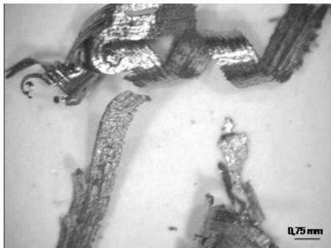
**Fig.9. Chips resulted at end-mill of sample 6**
