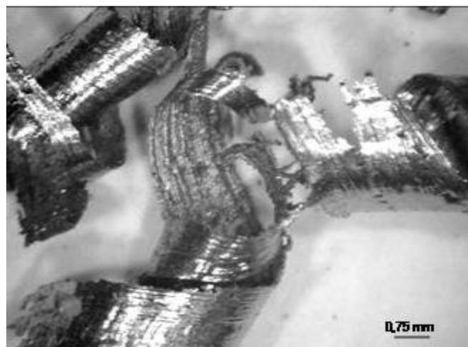
**Fig.5. Chips resulted at end-mill of sample 14**
