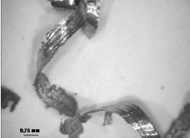
**Fig.18. Chips resulted after mill-end of sample 1**
