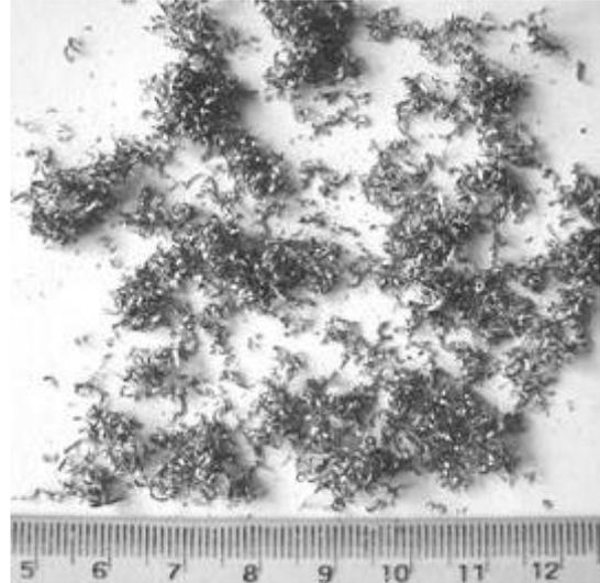
**Fig.19. Chips resulted after mill-end of sample 2**
