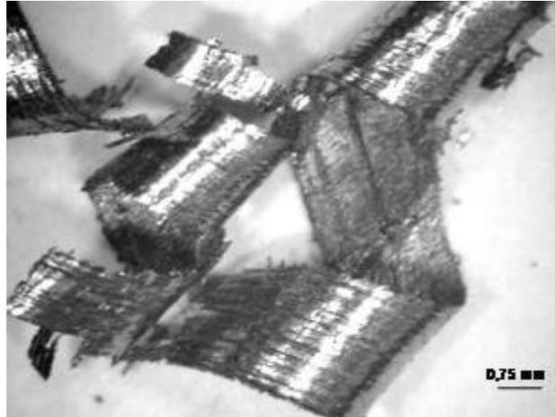
**Fig.7. Chips resulted at end-mill of sample 5**
