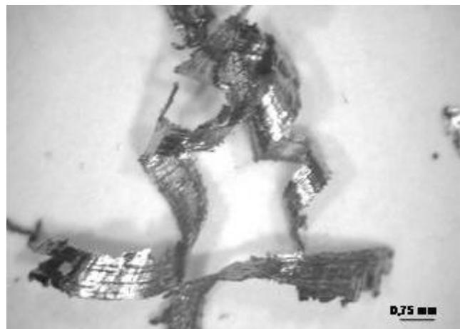
**Fig.13. Chips resulted after mill-end of sample 10**    **Fig.14. Chips resulted after mill-end of sample 11**
