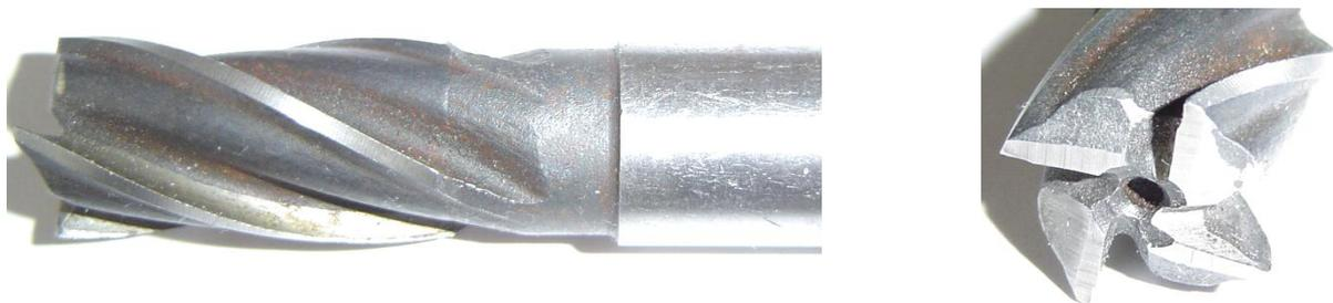
**Fig. 2. End-milling cutter used**
