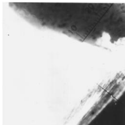
Fig.11. Deposits on cutting edge after turning with v = 625\text{m/min}
