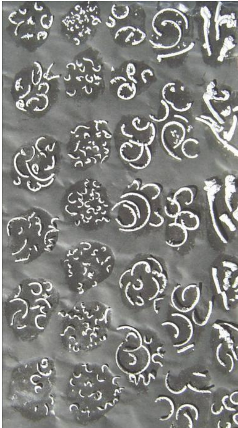
Fig. 1. Resulted chips after turning on different regimes
