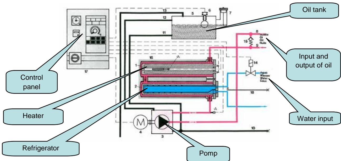
*Figure 2.2 Operating diagram of a thermoregulation unit*
