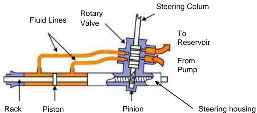
*Figure 1.1 The steering housing in assembly*
