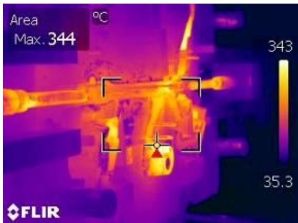
Mobile part of the mold before spraying
