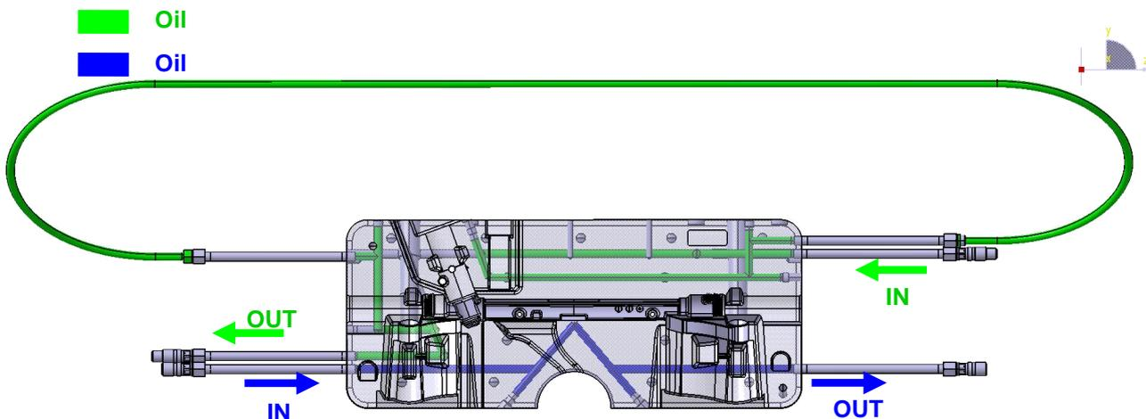
**Figure 3.2 Thermoregulation circuits with oil in the fix side of the mold**
