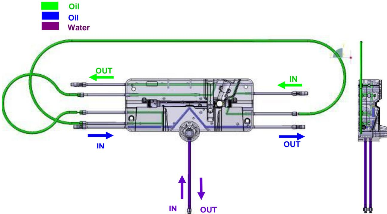
**Figure 3.1 Thermoregulation circuits with oil and water in the mobile side of the mold**
