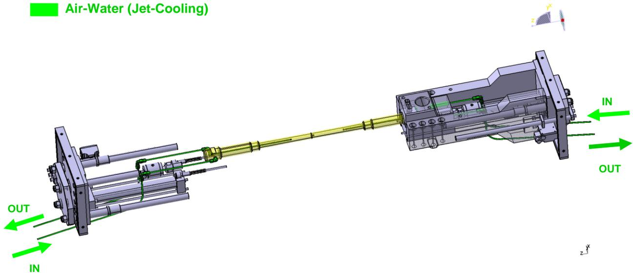
**Figure 3.3 Thermoregulation circuits of the pins with JET-COOLING system**
