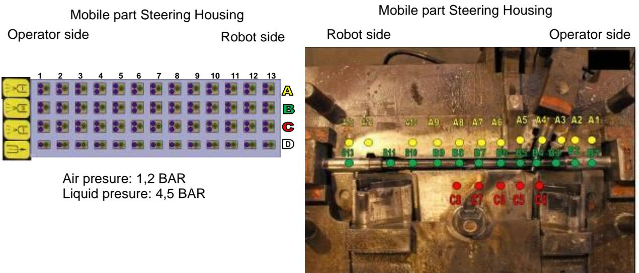
**Figure 4.2 Cooling-lubricating head for steering housing mold**
