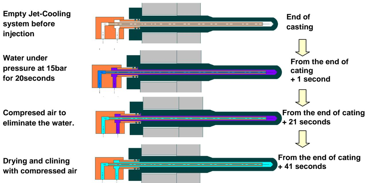
*Figure 3.5 Functioning of JET-COOLING system*
