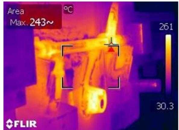
Mobile part of the mold after spraying
