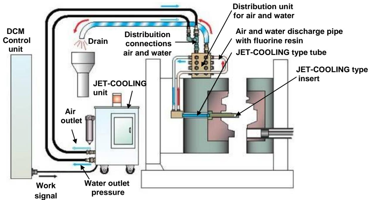
*Figure 3.4 Entire JET-COOLING system*
