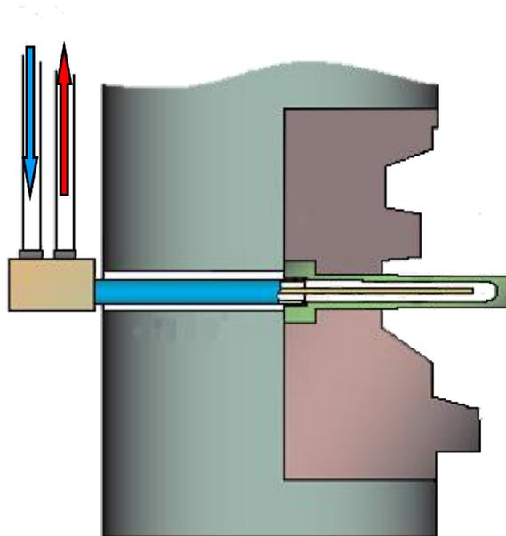
**Figure 3.3 JET-COOLING system in the mold**
